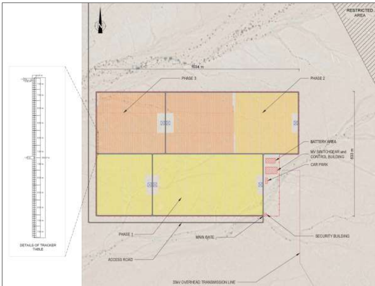
Figure 5-2: General Layout of proposed Gaingu PV Power Plant
