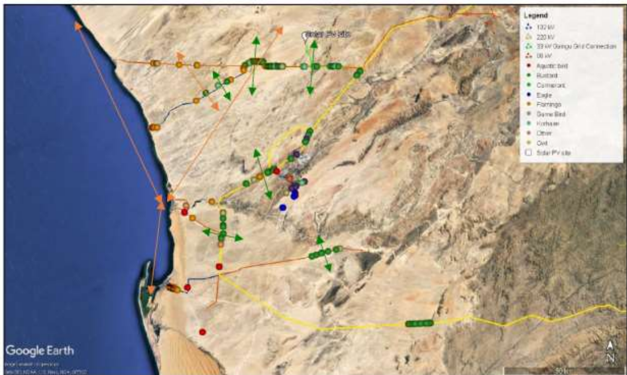
Figure 6-16: Power line incidents recorded within the Erongo Region, 2009-2020 (NamPower/NNF Strategic Partnership data; EIS 2023). Examples of bustard (and korhaan) flightpath areas (confirmed by power line collisions) are indicated by green arrows (note the variable directions of these paths); similarly, flamingo flightpaths are indicated by orange arrows (those along the coast have been confirmed by satellite tracking).
