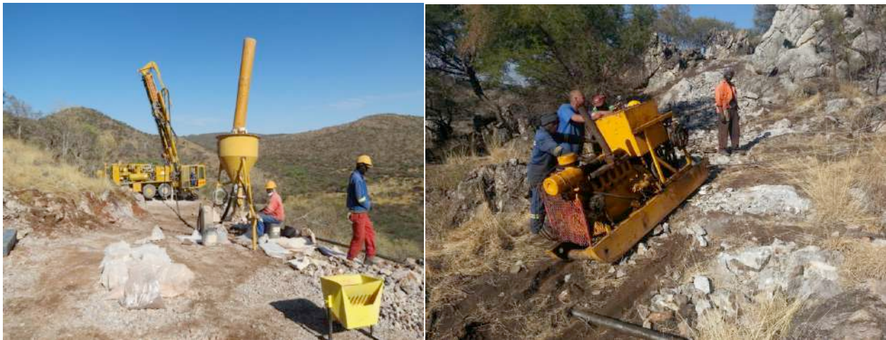
Figure 5. A truck mounted RC drill rig and a skid mounted drill rig (For illustration purposes)
