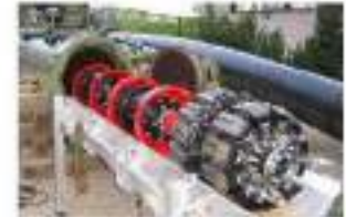
Intermediate lifting stations are installed at regular intervals.
