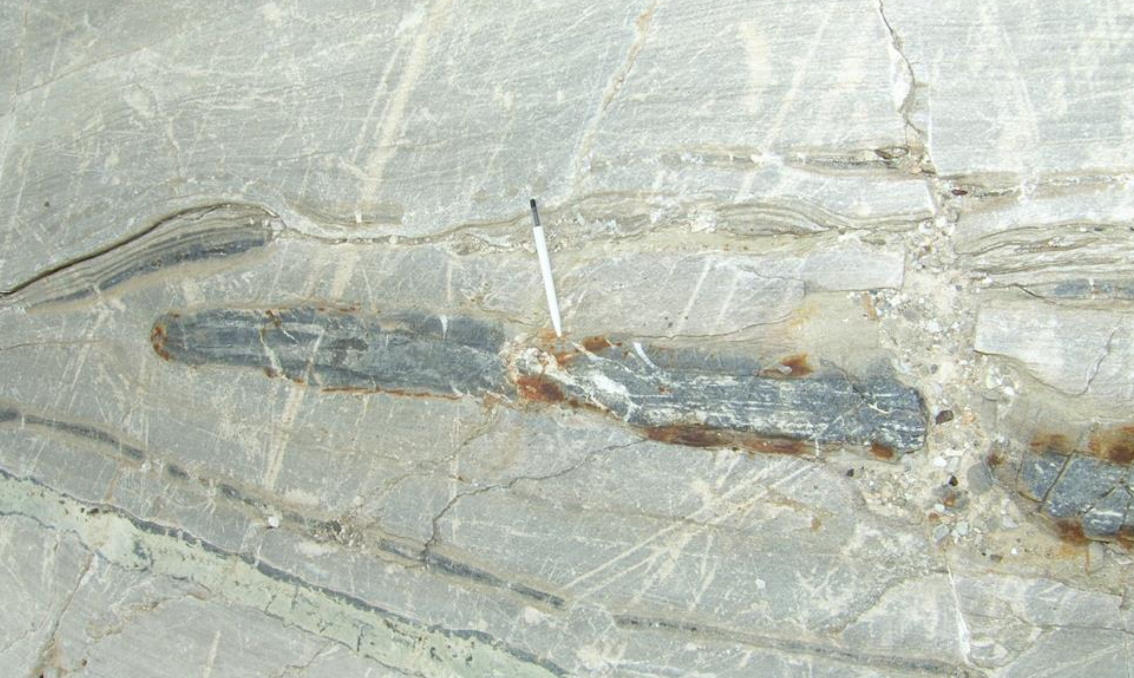
Plate 2.3: Impurities and discontinuities that must be removed from the marble blocks before transportation to the plant for final processing.
