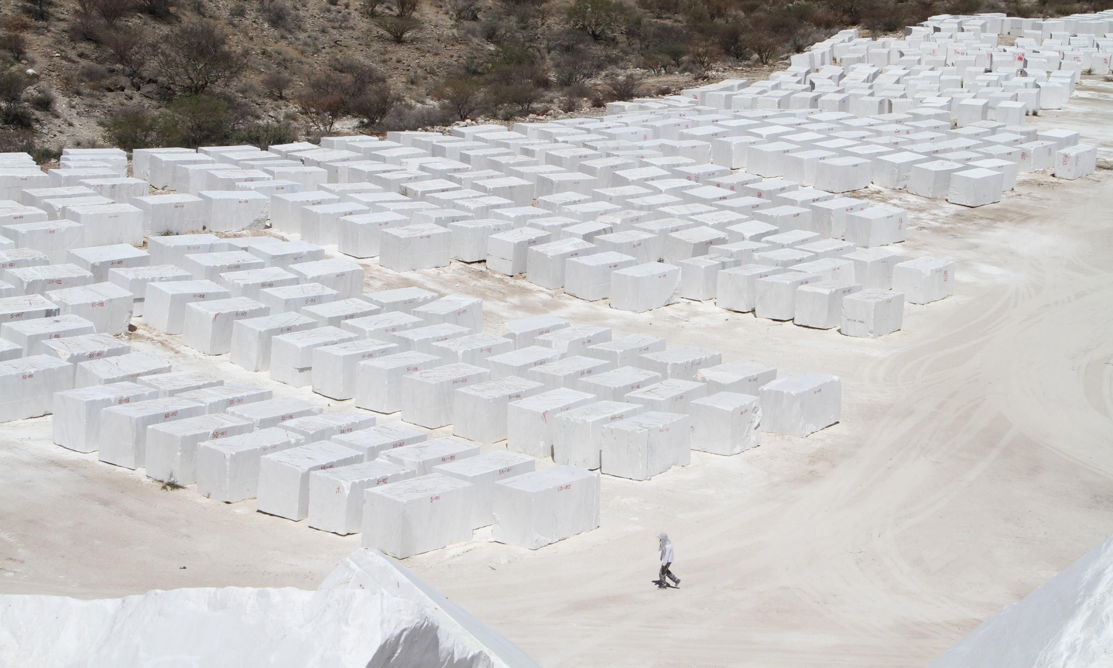
Plate 2.2: Mined blocks are stockpiled before sorting and transportation to the plant for final processing.
