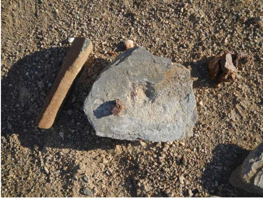
Site 293/510: Typical artisanal tin ore dressing assemblage with deeply dimpled mortar (schist) and pestle (columnar basalt) at left. The pestle is held vertically.
