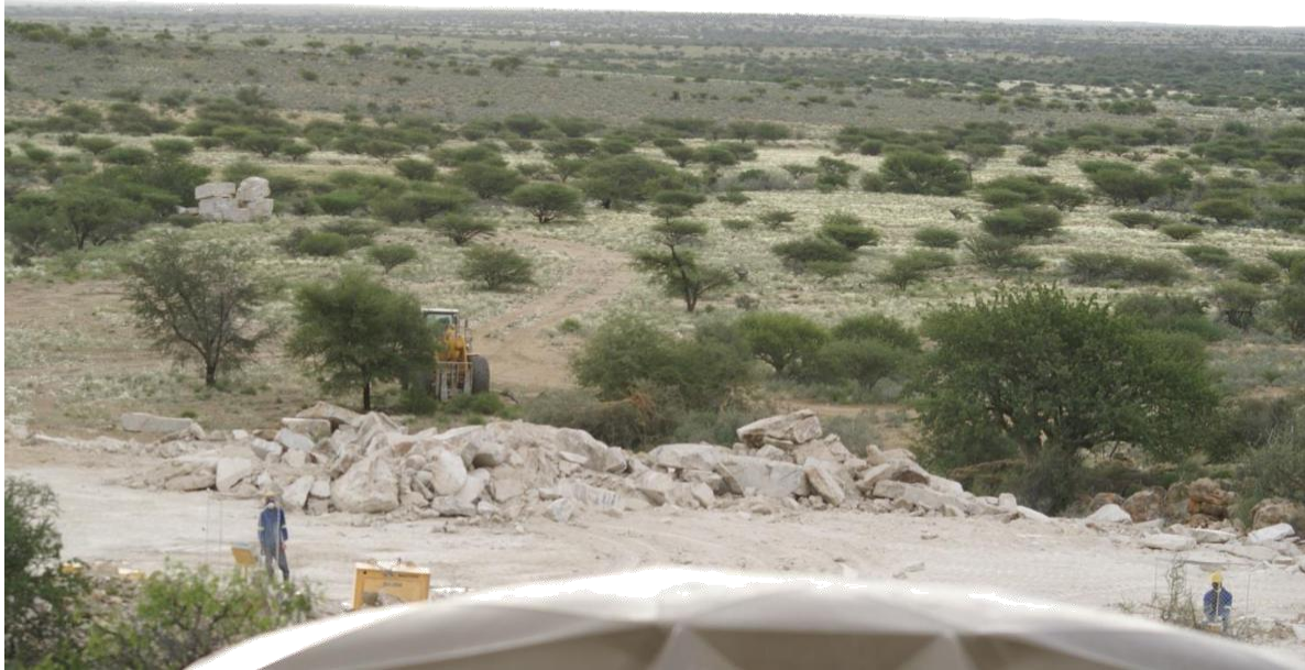
Fig 6 , Targeted Mining quarry outcrop in the Mining Licence, showing striped over burden during exploration.
