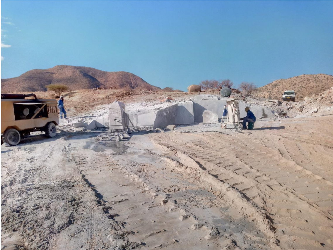
Fig 6 , Targeted Mining quarry outcrop in the Mining Licence, showing striped over burden during test mine.
