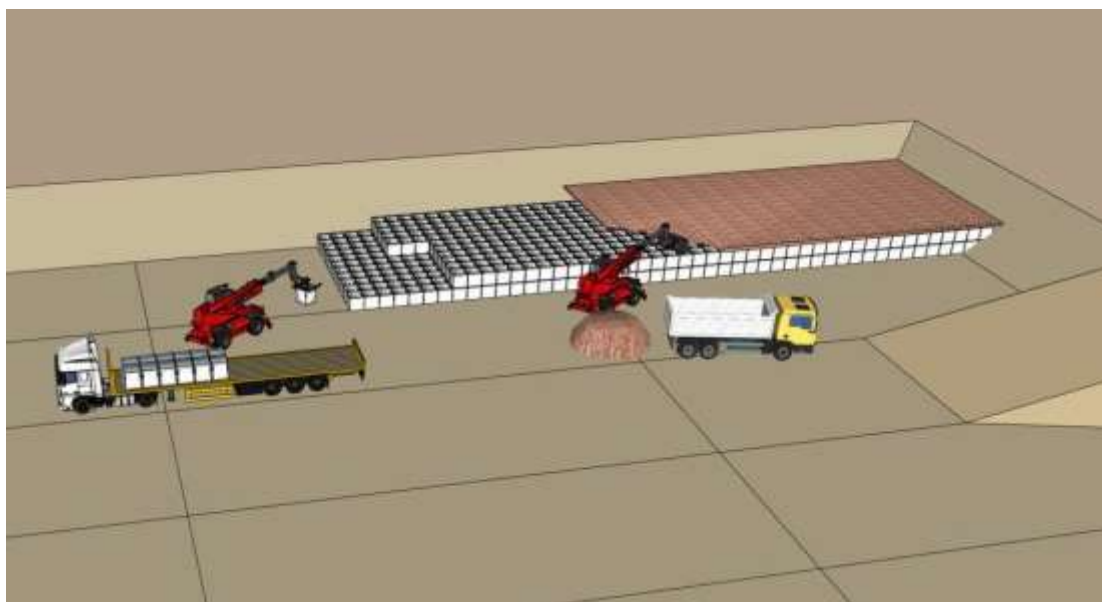
Figure 5-13: Filling of gaps between the big bags using sand.
