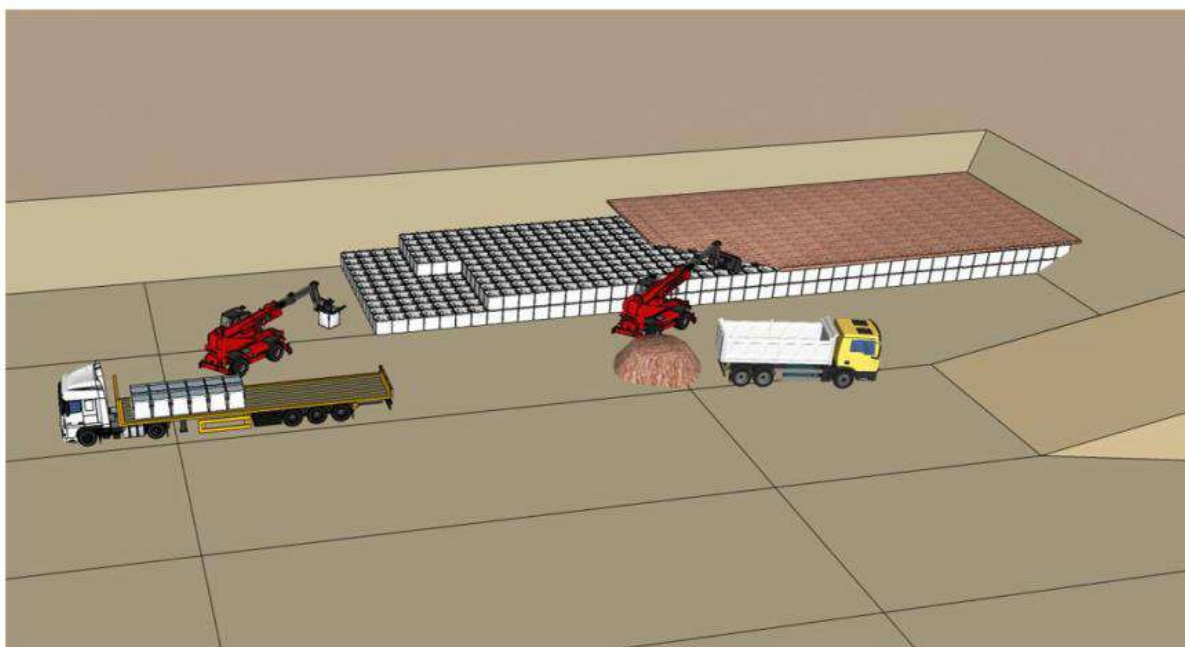
Figure 5-14: Filling of gaps between the big bags using sand.
