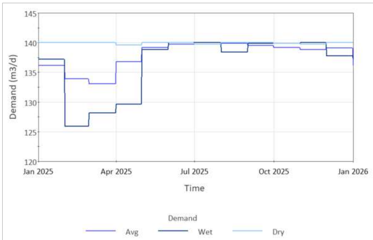
Figure 6-26: Total External Raw Water Demand (Phase 1A)
