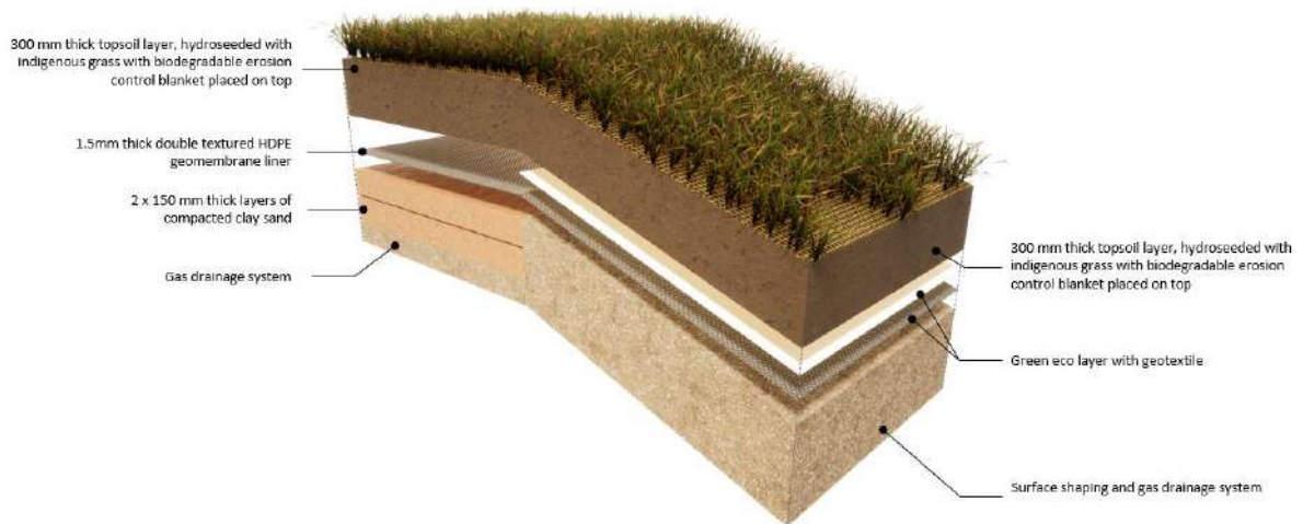
Figure 5-9: Typical capping system
