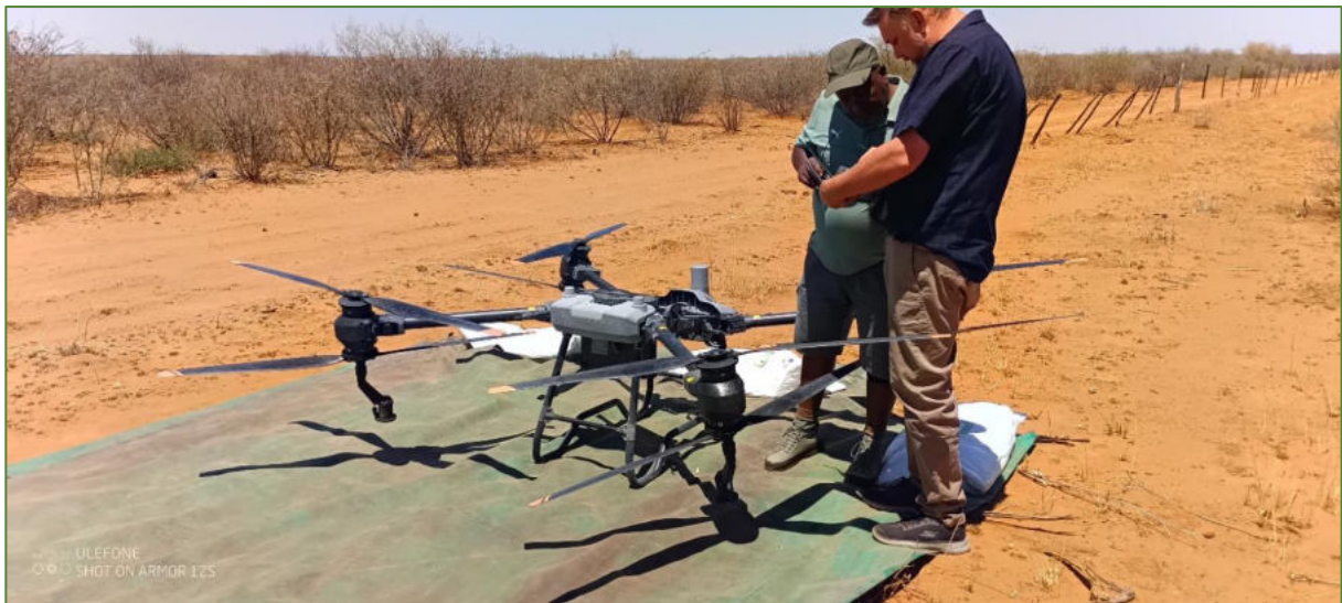
Figure 6: Illustration of the proposed drone obtained for the application of the herbicides, in the bag is the recommended Limpopo 200 GG Herbicides
