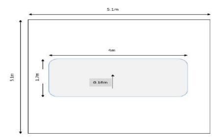
**Figure 3.1:** schematic pen layout with lengths and widths of the pen and pond, as well as the pond depth. **NOT TO SCALE.**
