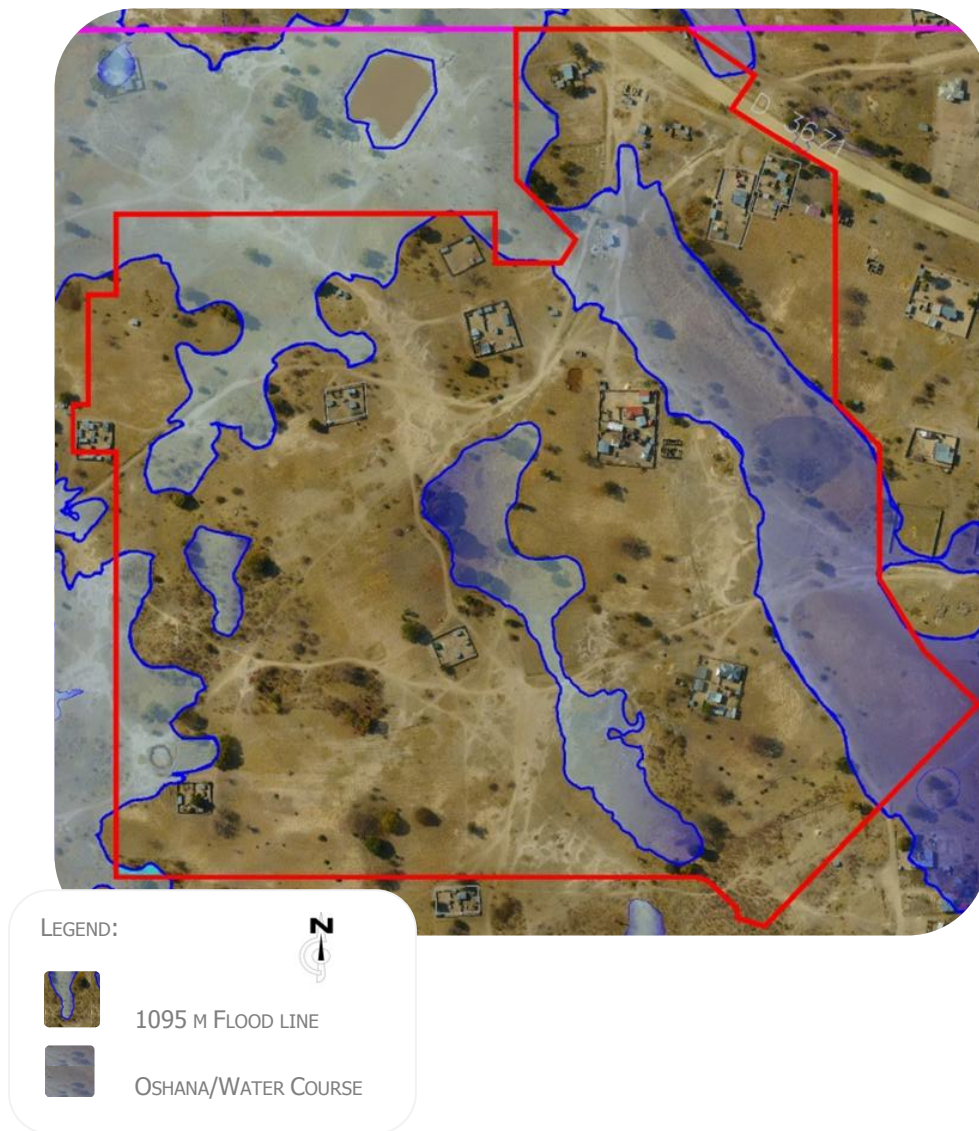
Figure 7: 1095 m Flood line on the site
