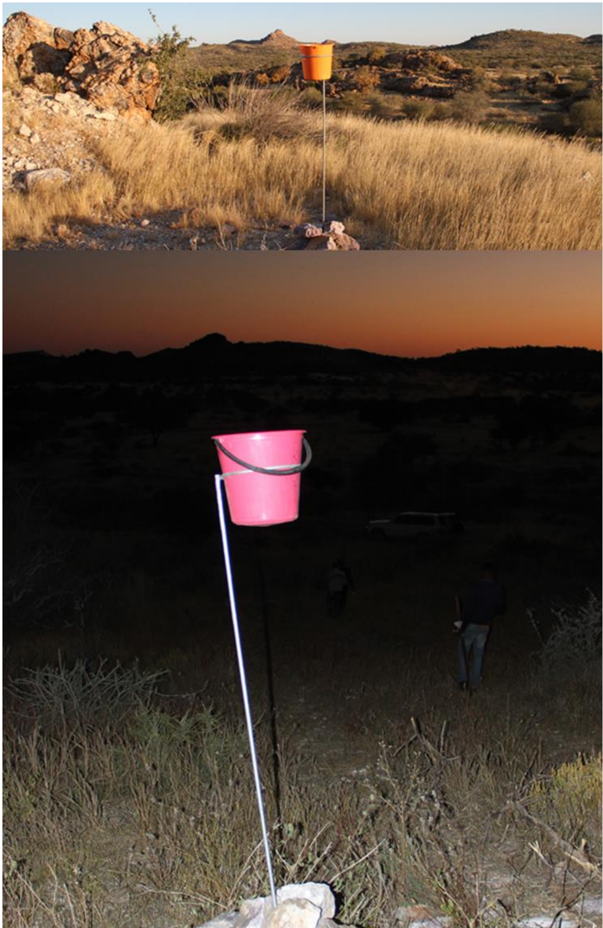
Plate 4.1: Dust monitoring stations to be established within the ML 205 as part of the monitoring programme (RBS Geotagged Image Series, 2017).
