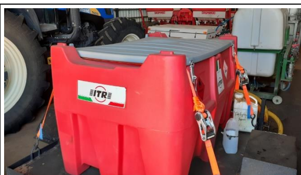
Photo 4-15. Mobile Diesel tank
