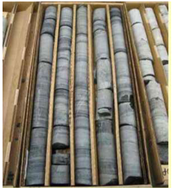
Figure 12: Core Sample – Granite Rock
