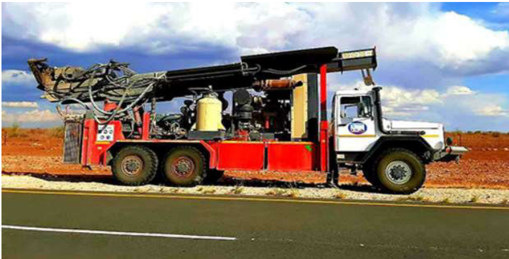
Figure 6: A Typical Drill Rig Truck (Source: African Drilling)
