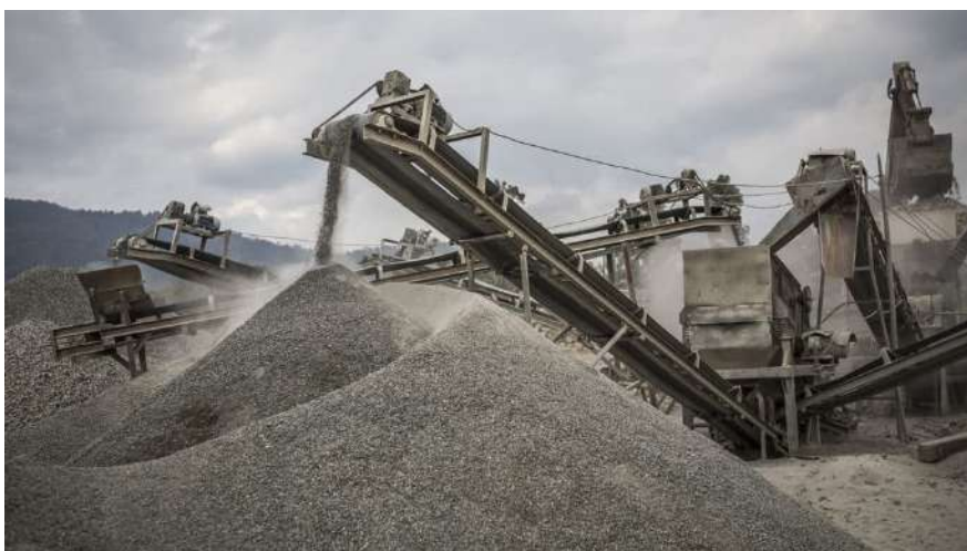
Figure 6. Stockpiling of aggregate
