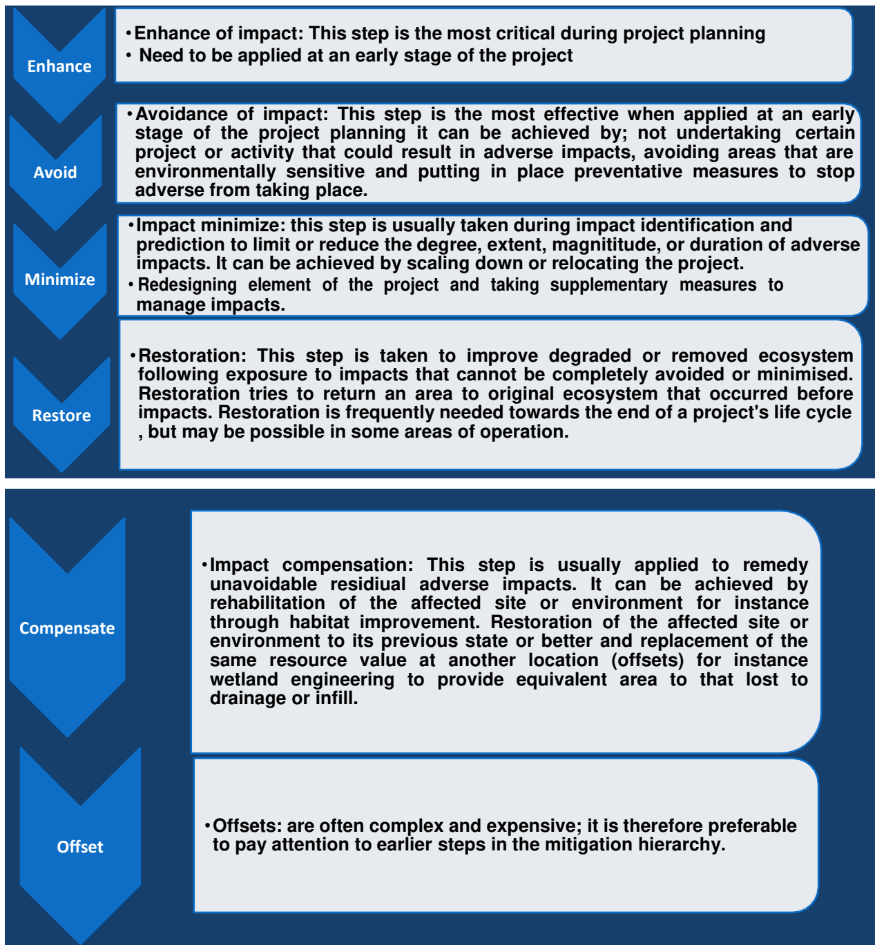
Figure 12: The mitigation hierarchy of action used to retort to any proposed project or activity.
