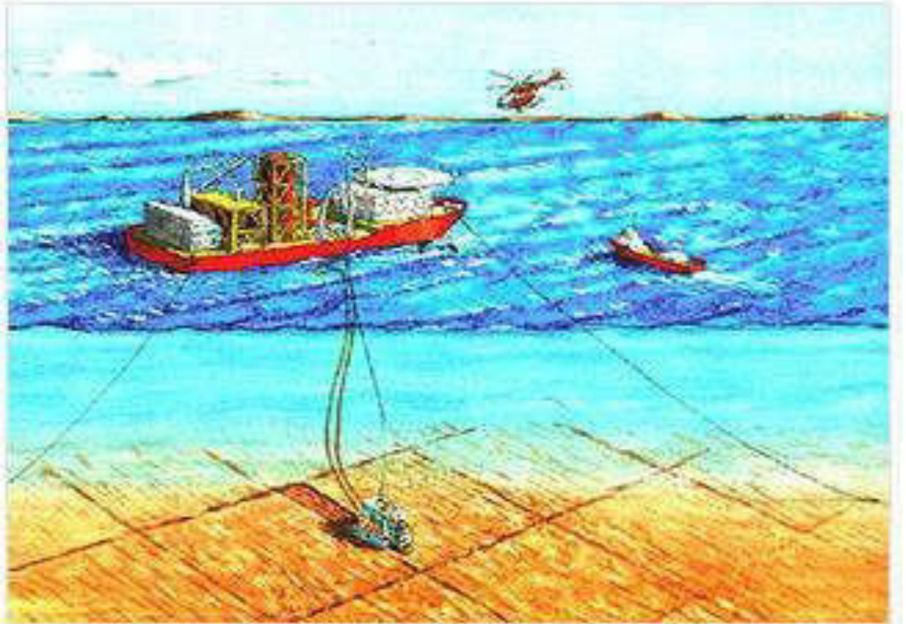
Figure 4: Depict the airlift drilling technology to be used for diamond exploration on the seabed at EPL 8627.
