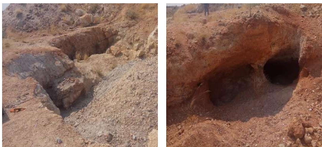
Photo 16: Open excavated trenches – unrehabilitated and unfenced
