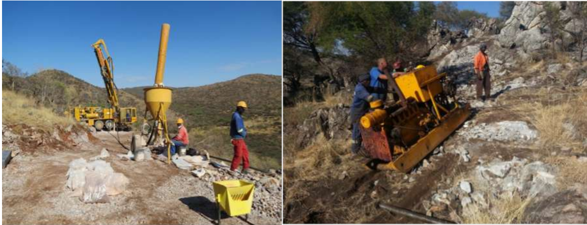
Figure 6. A truck mounted RC drill rig and a skid mounted drill rig (illustration only)
