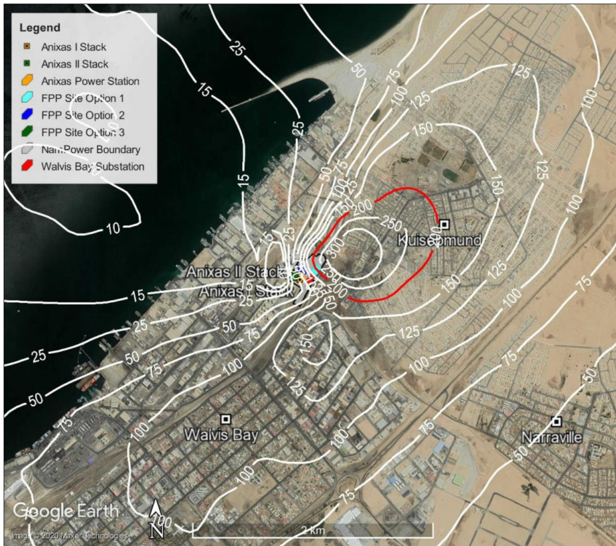
Figure 5-10. Predicted 99 th percentile of the 1-hour NO 2 concentrations in µg/m 3 for Scenario 4 (uMoya-NILU, 2020)
