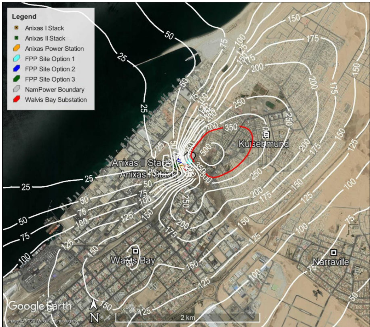
Figure 5-7. Predicted 99 th percentile of the 1-hour SO 2 concentrations in µg/m 3 for Scenario 2B (uMoya-NILU, 2020)
