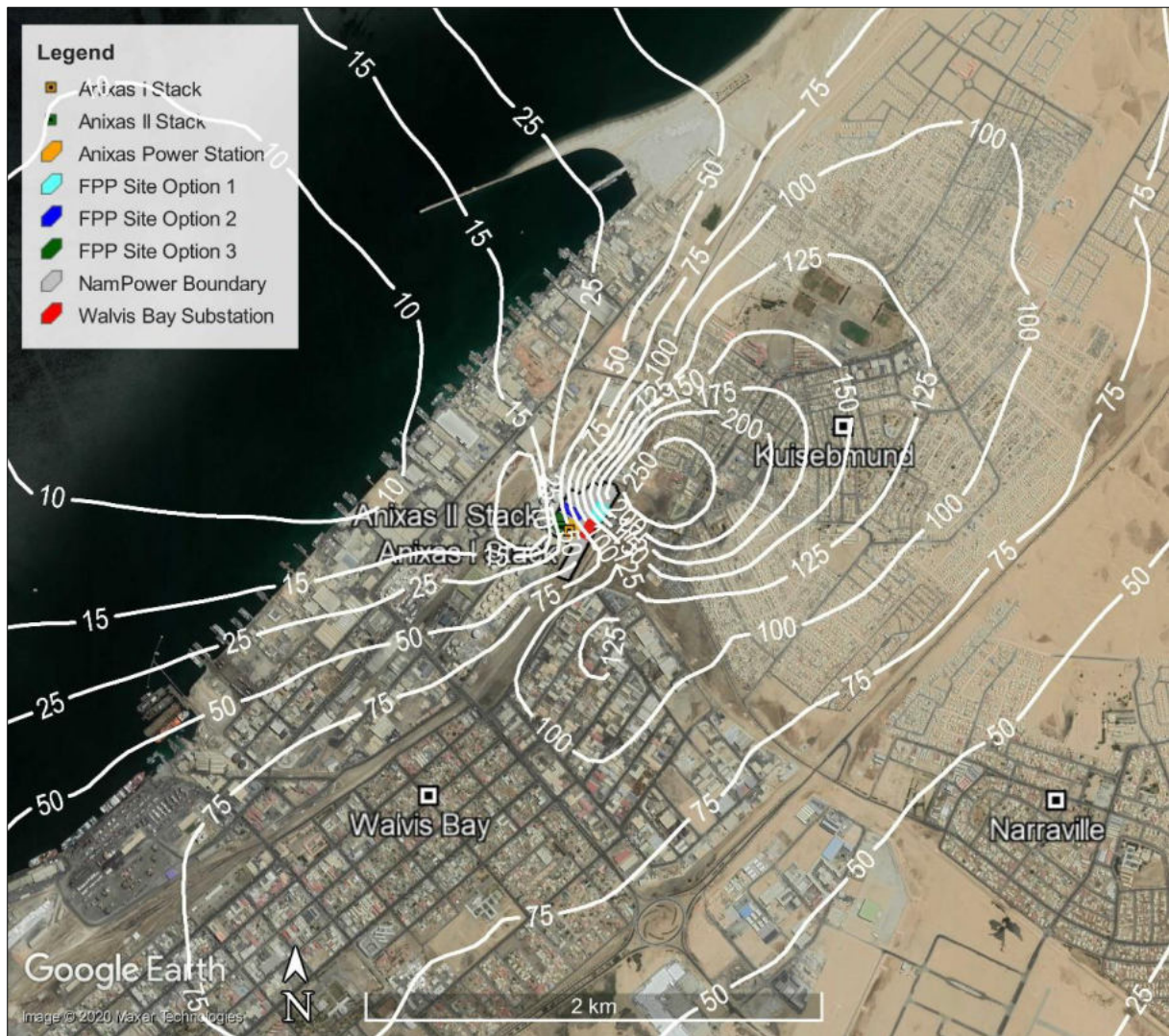
Figure 5-11. Predicted 99 th percentile of the 1-hour SO 2 concentrations in µg/m 3 for Scenario 4 (uMoya-NILU, 2020)
