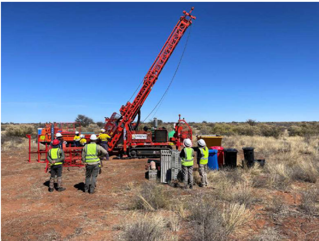
Figure 18 - Diamond core drill rig utilised for the drilling programme activities (Source: RES)
