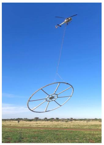
Figure 3 – AEM survey in operation, on take-off Kiripotib airfield (Source: Proponent)
