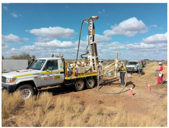
Figure 4 – Air core drilling rig in operation during activities on EPL 7528 (Source: Proponent)
