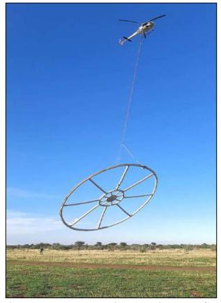
Figure 3 - AEM survey in operation, on take off
