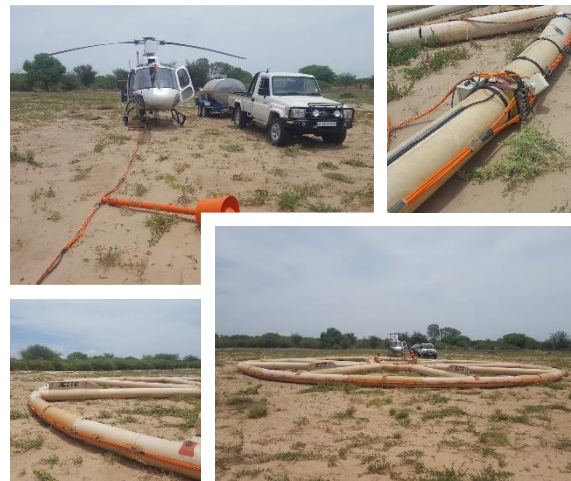
Figure 3-2: Airborne geophysics instruments
