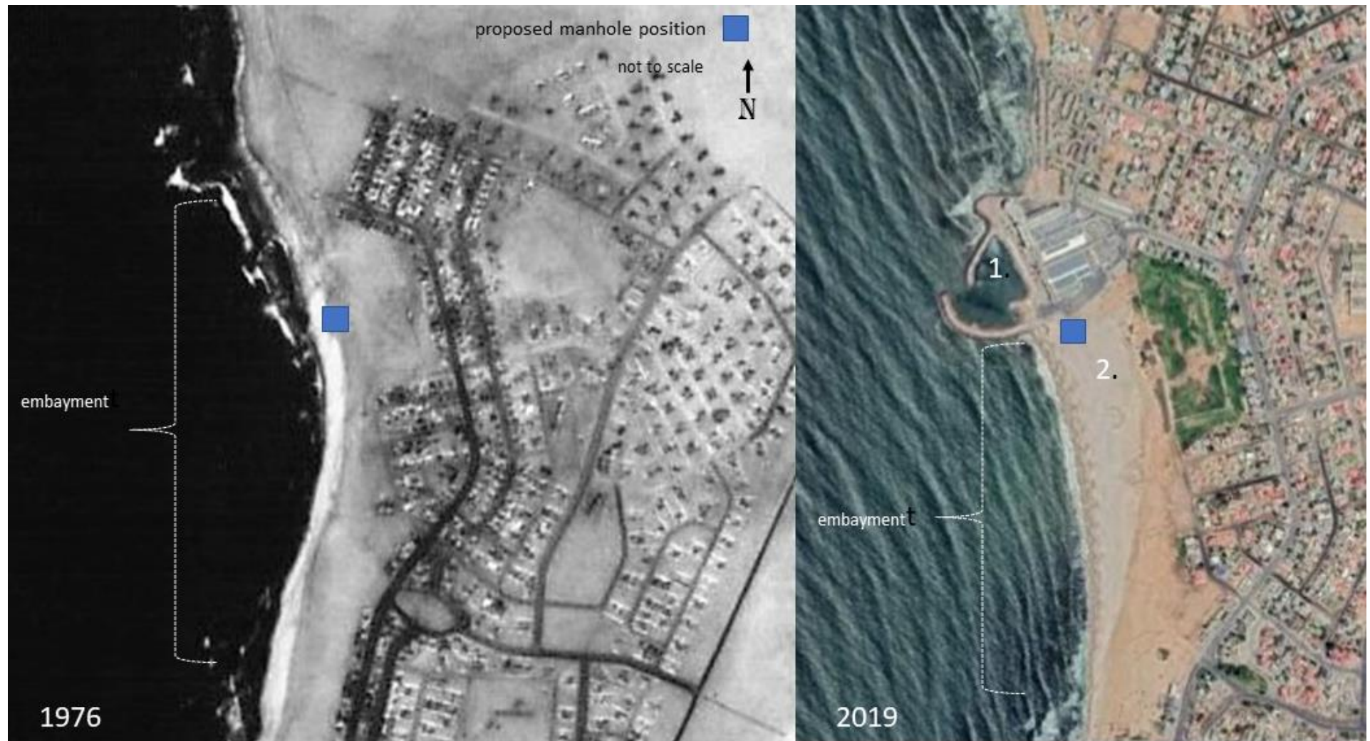
Figure 6. Comparative aerial imagery of site from 1976 and 2019. Note approximate position of manhole for cable landing point and 1. presence of harbour and 2. expansive or widening beach environment.
