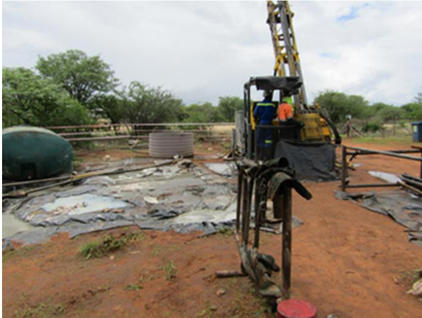
Figure 2 - Plastic lined sumps and drilling in progress
