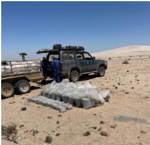
Figure 3 - Sample bags and material from drill hole used to refill holes for rehabilitation
