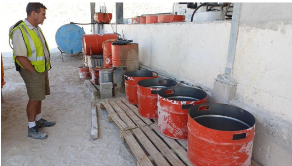
Photo 10 – View of experimental area where sawdust is used to clean polluted soil.
