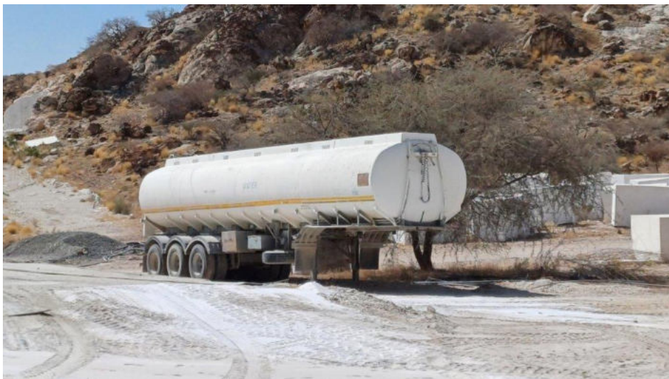
Photo 24 - View of water tanker with which water is transported to site.
