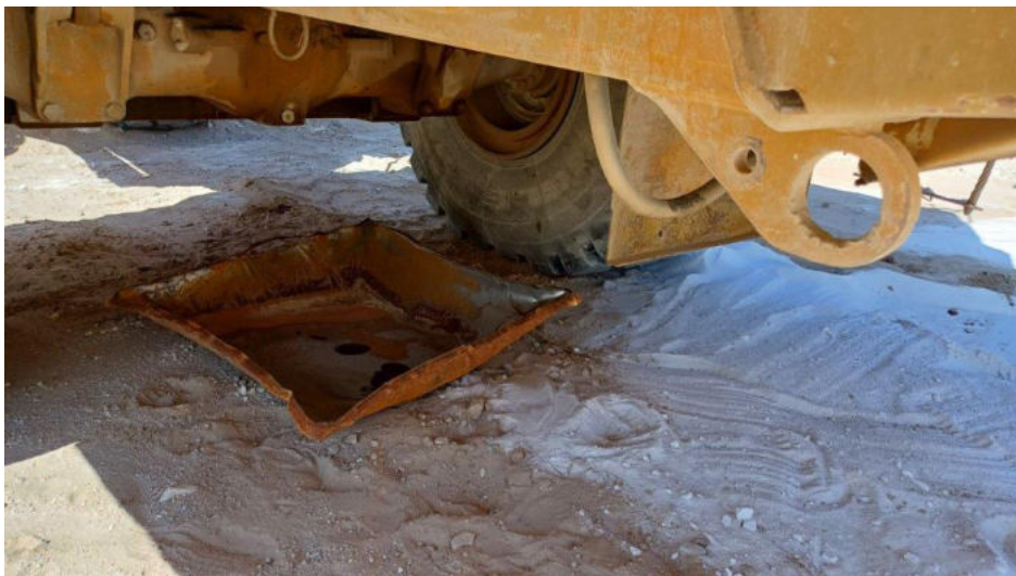
Photo 22 – View of drip tray underneath a stationary construction vehicle.
