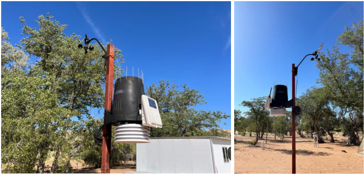
Figure 10 - Vantage 2 pro weather station at Lofdal camp
