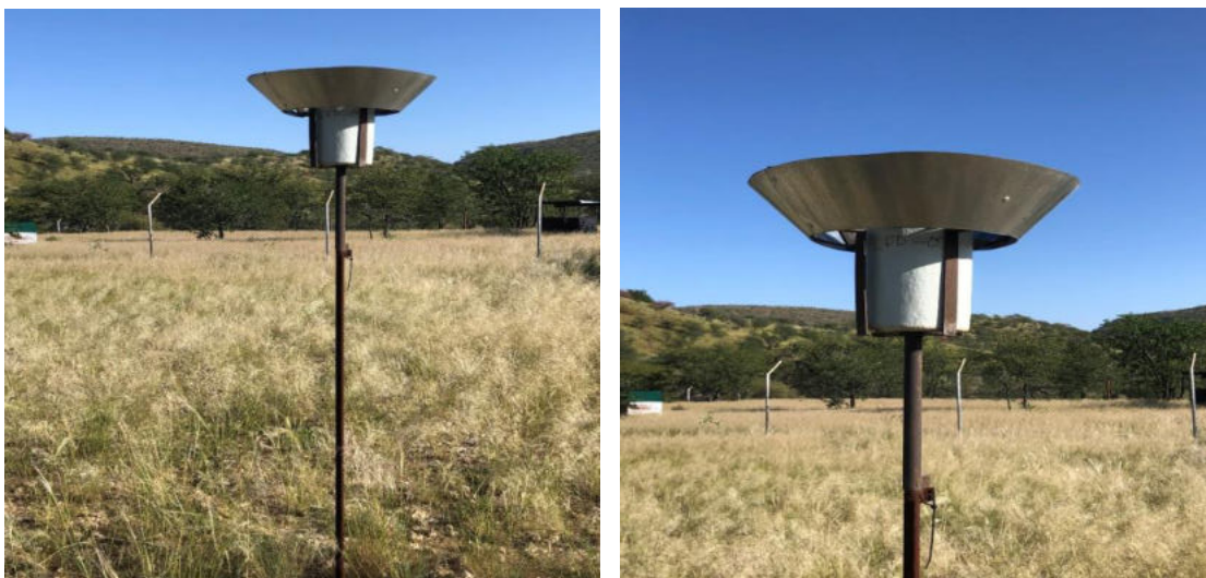
Figure 9 - Dust Fallout Unit (LFD 01)
