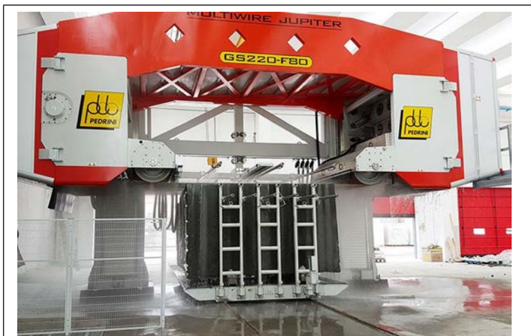
Photo 3.1 – View of diamond multiple-wire cutting machine
