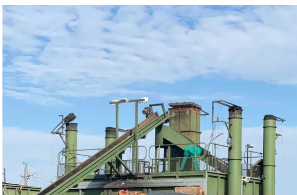
FIGURE 4 - VIEW OF THE RETORT KILNS ON SITE IN OPERATION. NOTE: NO VISIBLE EMISSIONS WHEN THE KILNS ARE OPERATED CORRECTLY
