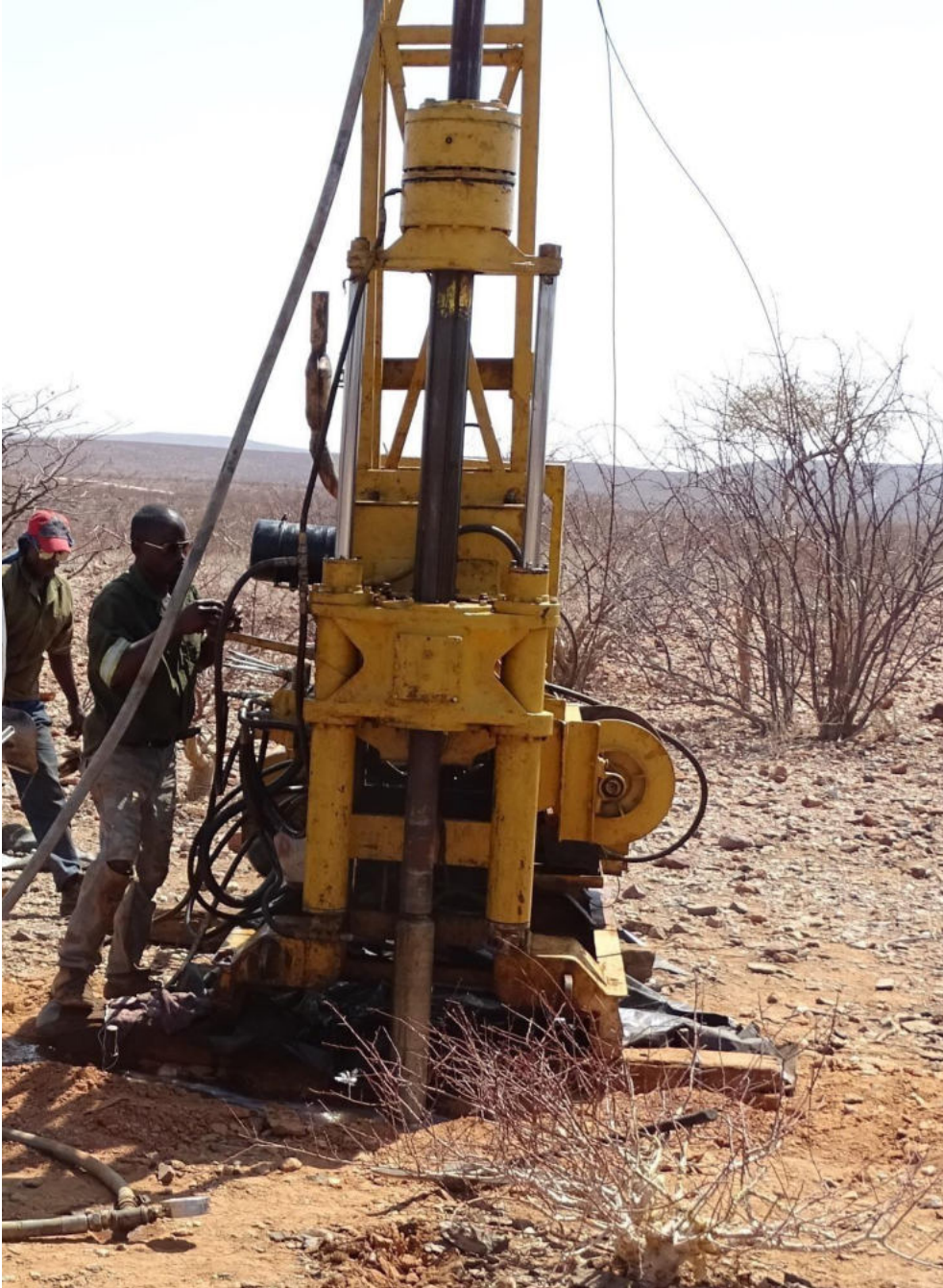
Fig 4... Showing the rig that was used during diamond core drilling.
