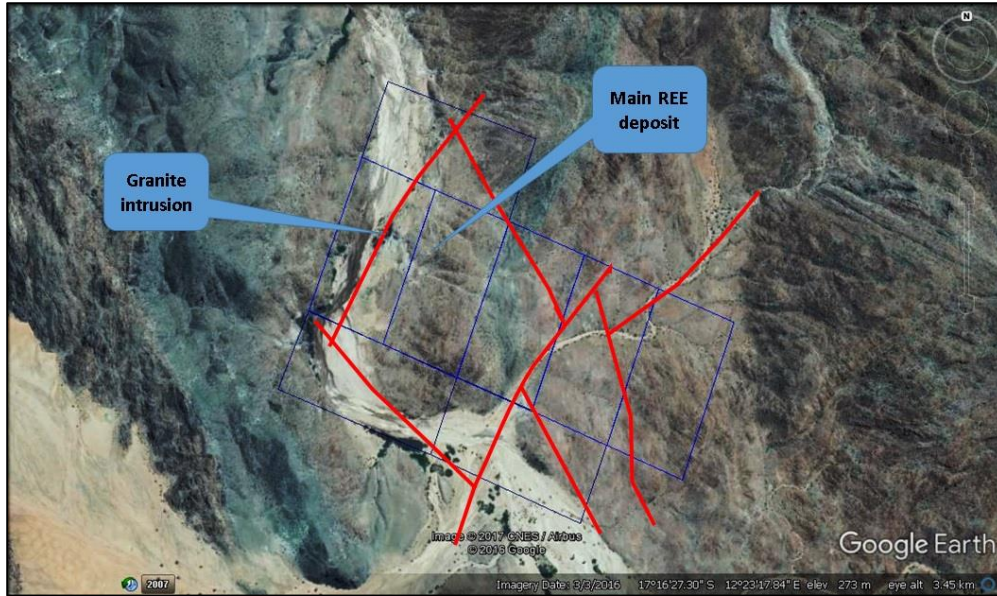
Fig. 5. Uplifted tectonic block with REE deposit constrained by numerous faults.
