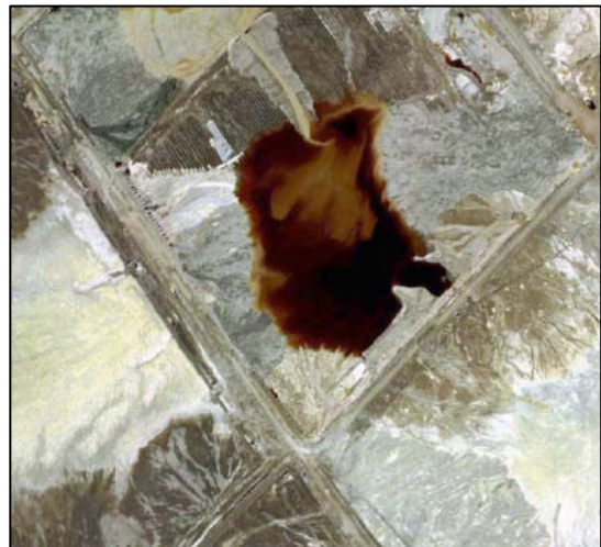
Figure 19: Tailings paddocks showing grey and yellow chemical precipitates after dessication (source: RUL)
