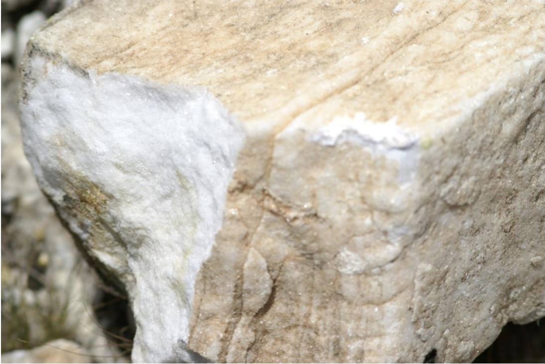
Figure 4: Homogeneous marble within the in MENETTE NYEUDO HAIPINGE MINING CLAIMS as seen in a hand specimen
