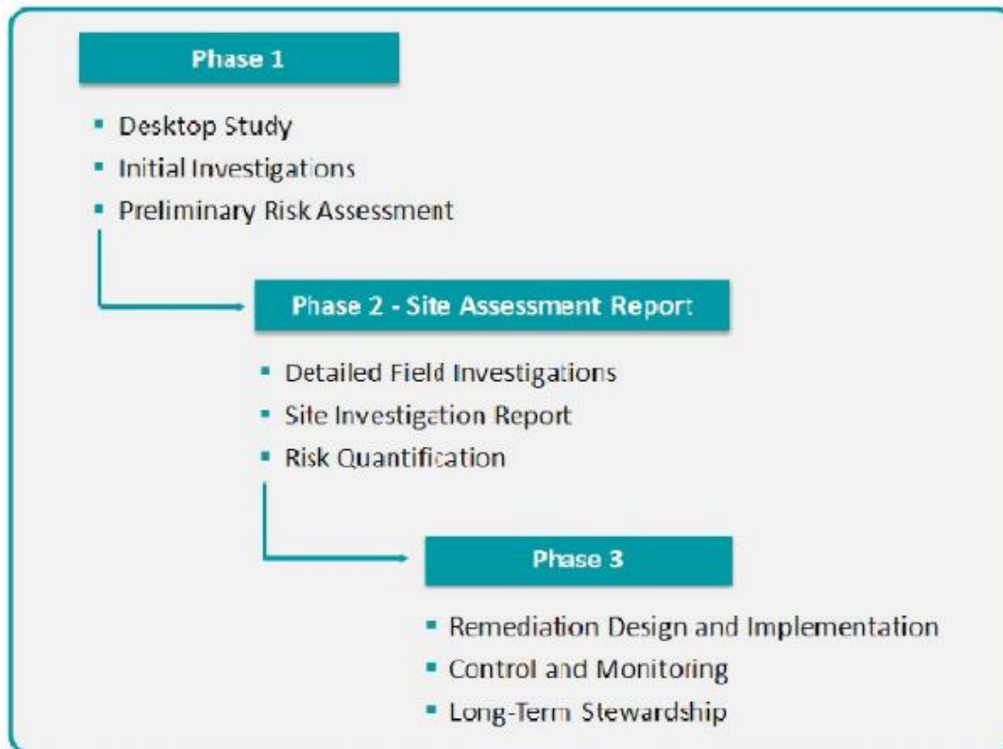
Figure 31: A phase approach for the assessment and remediation of contaminated land (Ashraf et al. , 2014)
