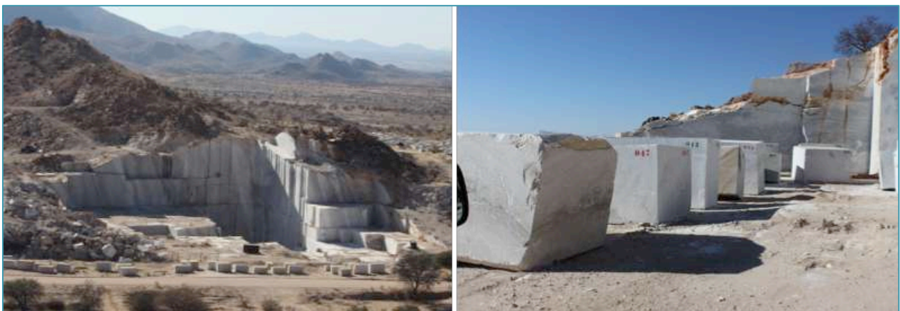
Fig 11: Shows general setup of a marble quarry where block are extracted and stored before being hauled to the harbour town for shipping (this is the least radioactive quarry activity).
