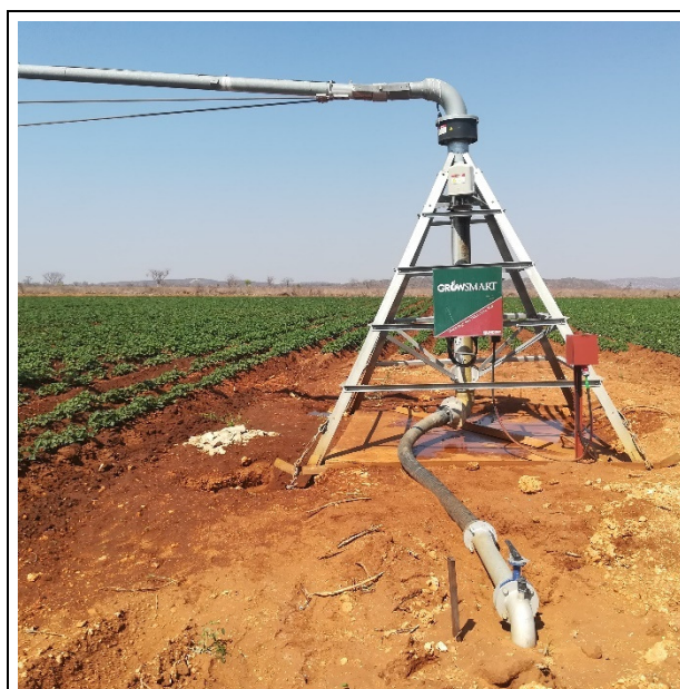
Photo 4-11. Typical Center Pivot System with Fixed Central Tower (Phocaides (2007))
