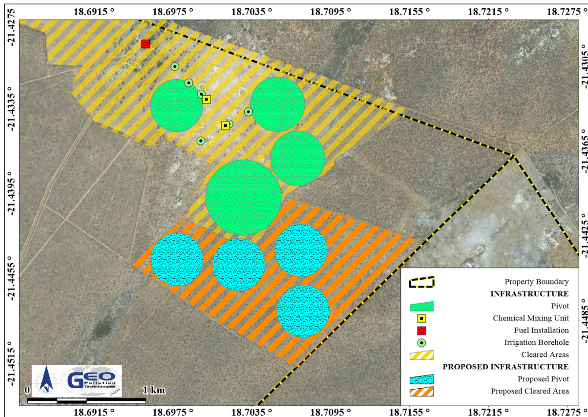
Figure 4-2. Irrigation and infrastructure layout on the Farm Okasondana
