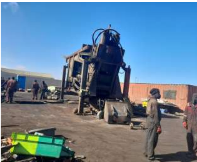
Photo 3. The baling machine used to cut scrap metal. Photo 4. The baling machine for compacting and shredding
