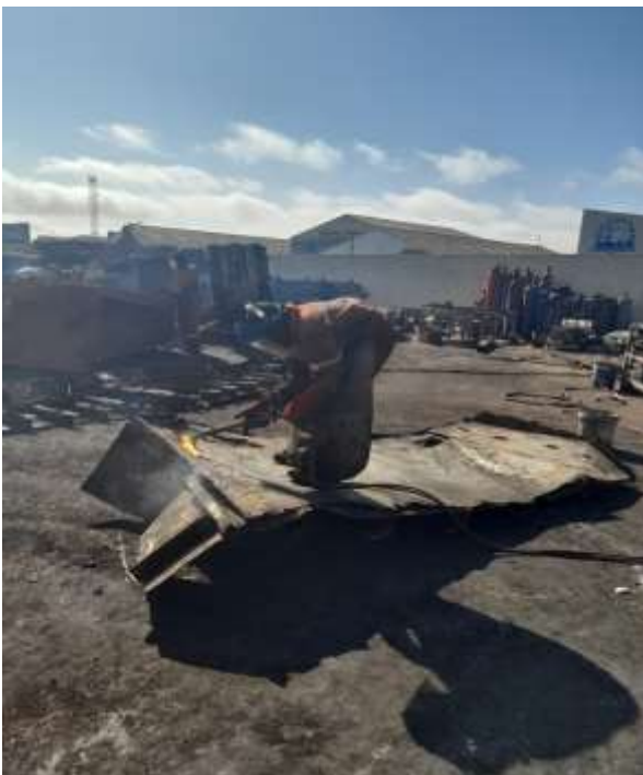
Photo 5. Workers cutting scrap metal using flame torch. Photo 6. Gas bottles use and storage
