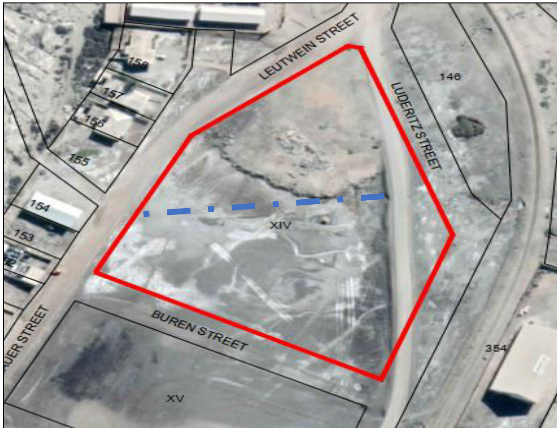
Figure 16: Estimated alignment of the sewer line
