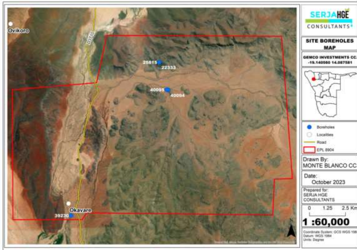
Figure 5-17: The existing water boreholes within the EPL boundaries
