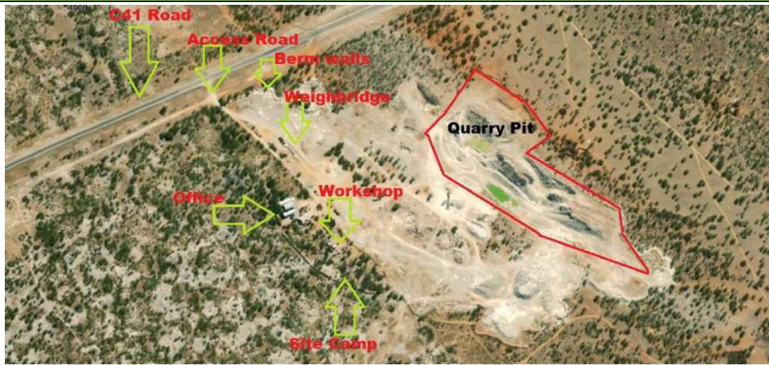
Figure 3: Quarry Layout & Facilities
