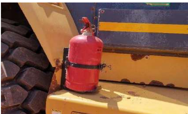
Figure 27: Fire extinguisher - earthmoving truck
