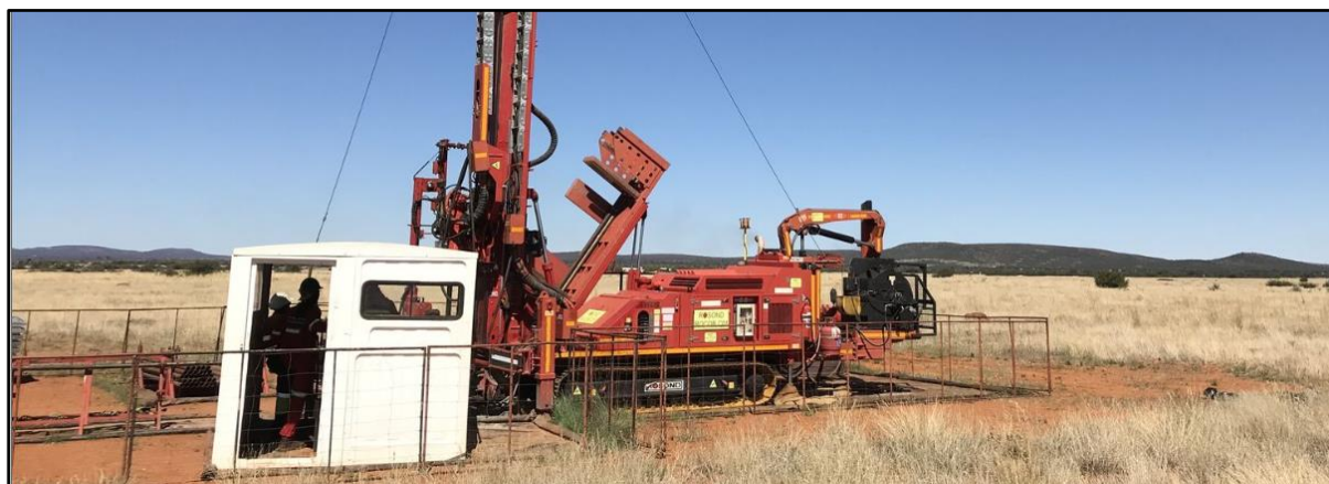
Figure 4: A typical example of a Down-The-Hole drill rig
