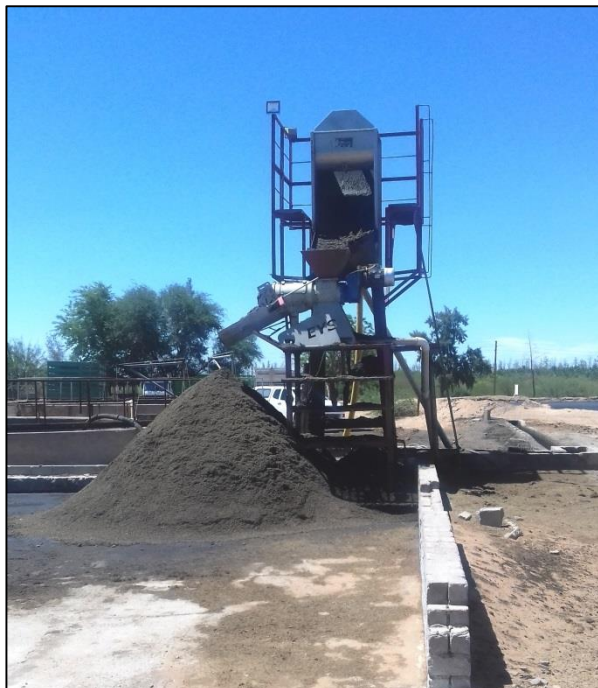
Picture 4: Manure removed from slurry using a separator
