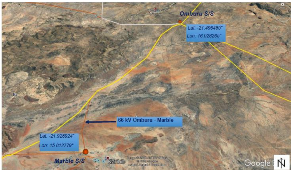
Figure 1: Map showing the 66 kV Omburu – Marble transmission line
