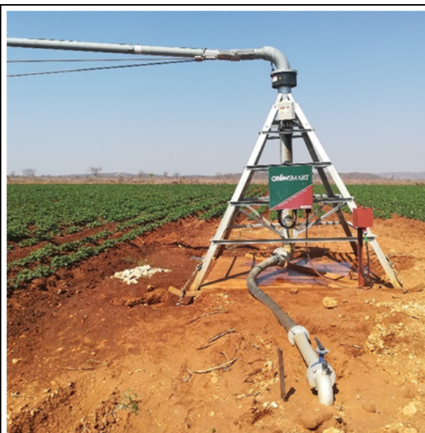
Photo 4-7. Typical Centre Pivot System with Fixed Central Tower (Phocaides (2007))
