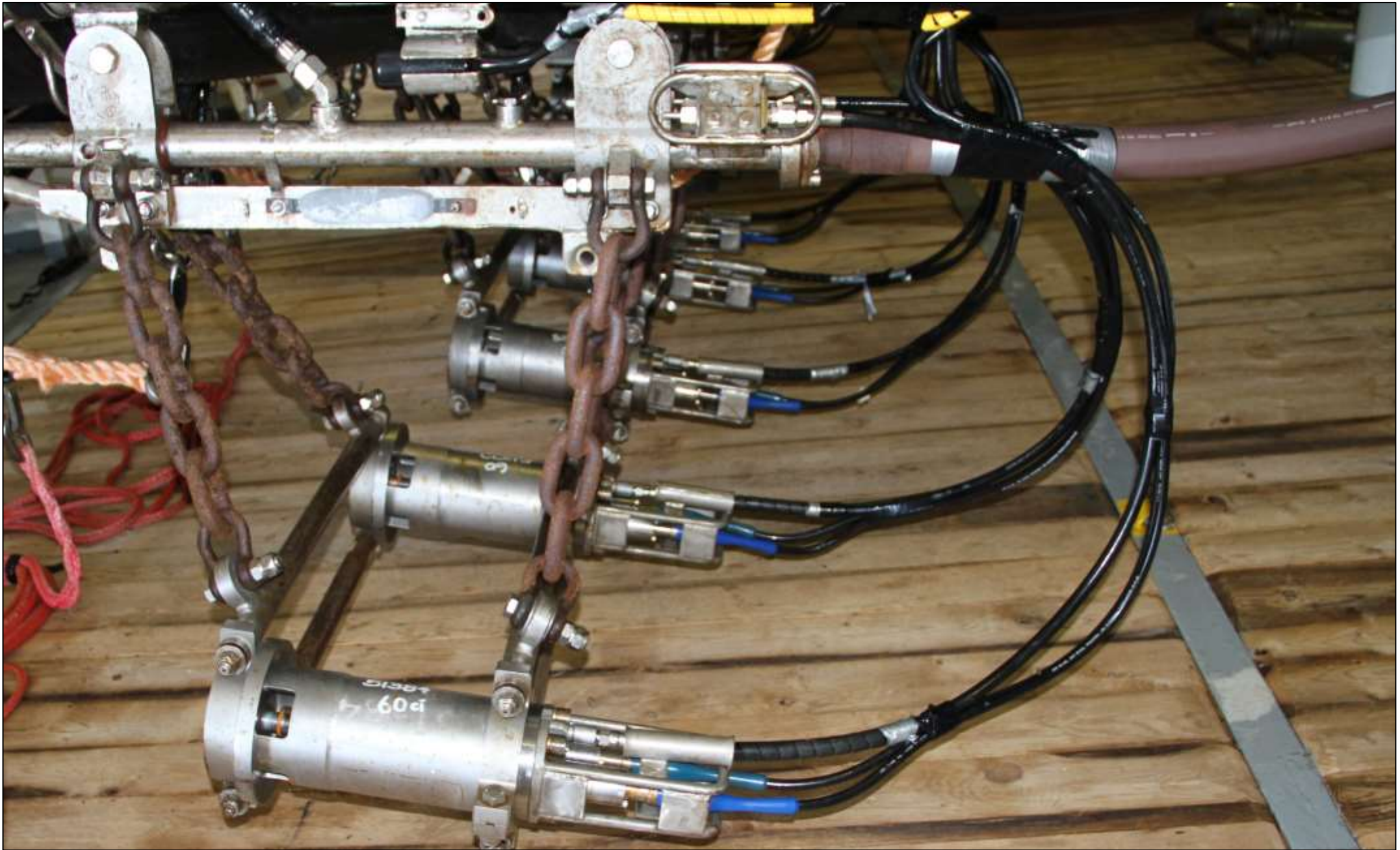
Plate 2.1: Example of the air guns used in marine seismic survey operations.
