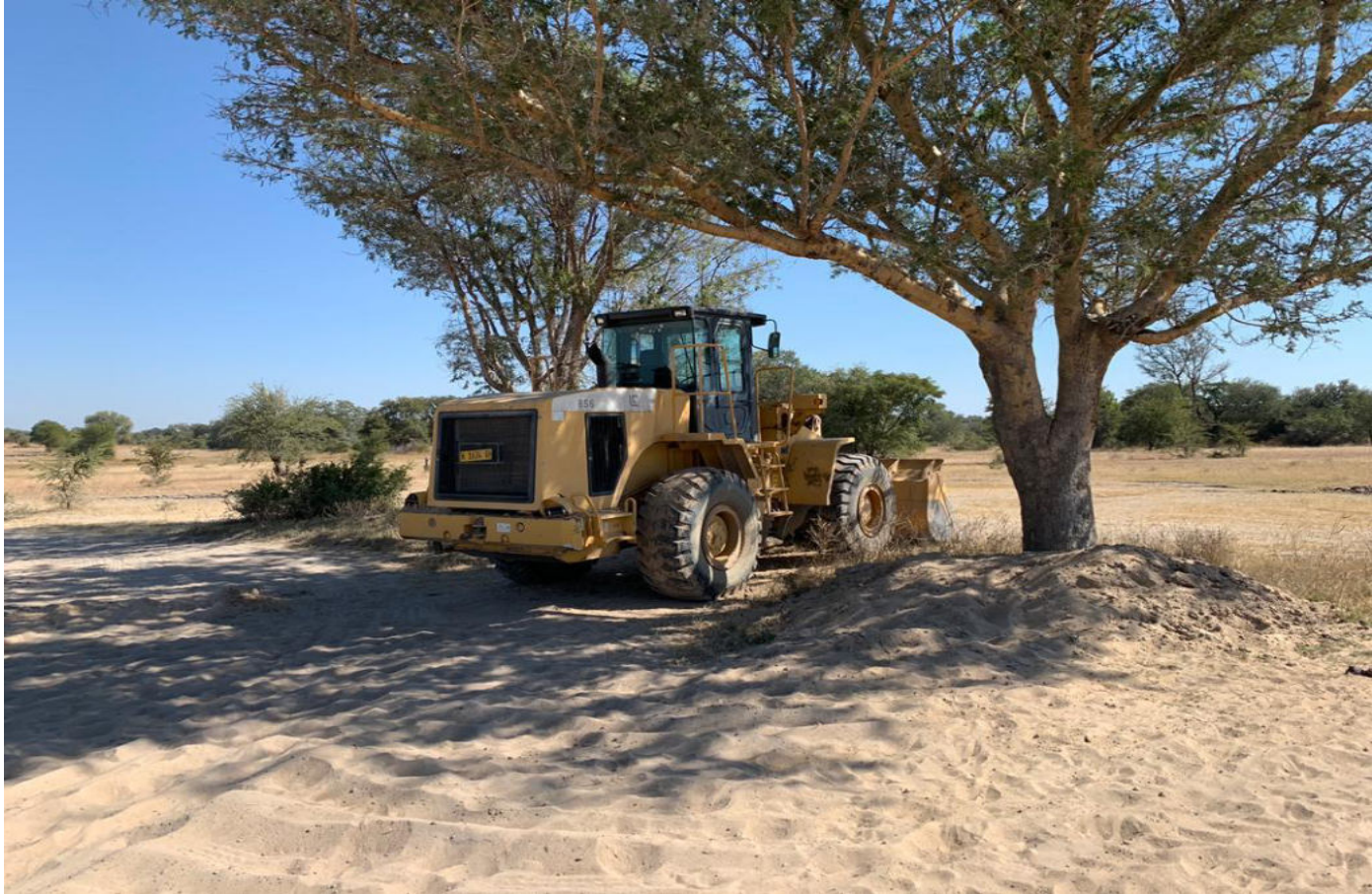
Sand mining equipment front-end loader
