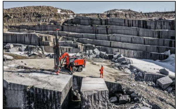
Down-the-Hole drilling (applied in mining)
