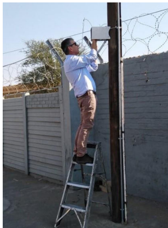
Figure 4: Setup of the Meatco Radiello™ passive diffusive tubes
