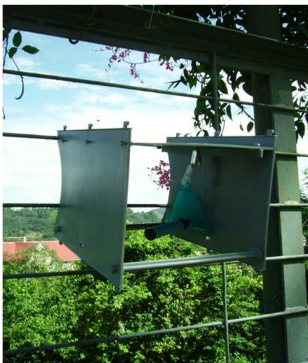
Figure 3: Typical setup of Radiello™ passive diffusive tubes
