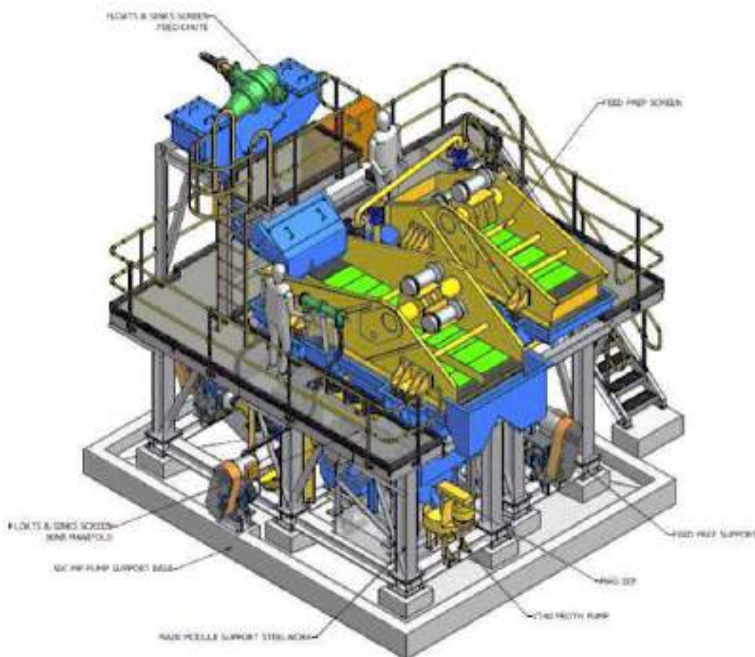
Figure 18 - Schematic diagram of the petalite beneficiation plant
