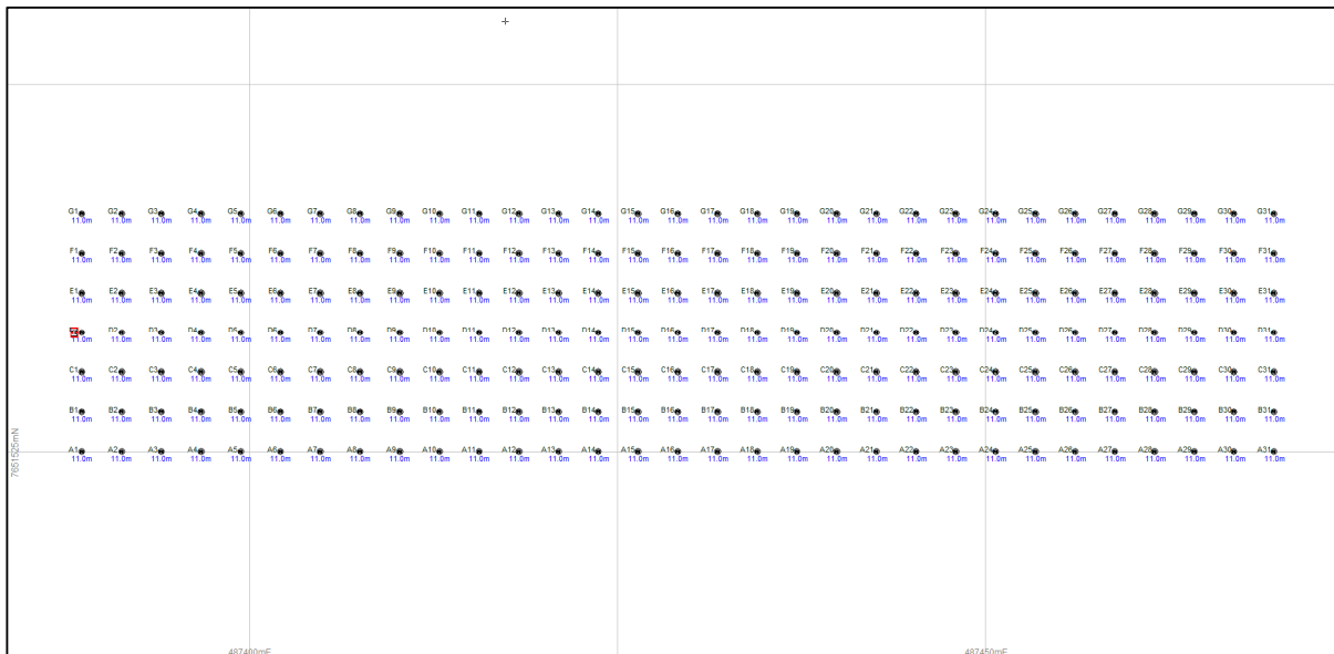
Figure 9: Blast Area with blastholes and depths
