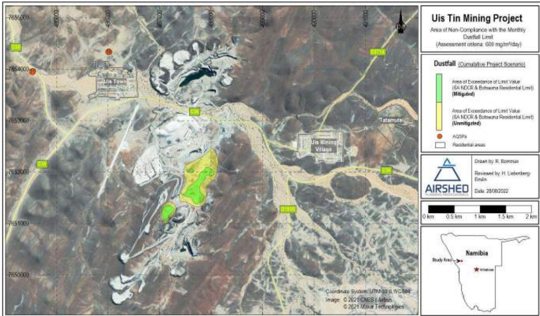
Figure 39: Area of non-compliance with the monthly dustfall AQO for unmitigated and mitigated cumulative Project operations
